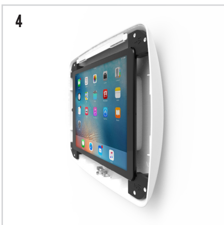
4 Place the tablet into the case and plug in the power cable.
