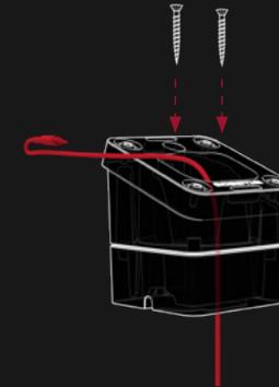
4. With the cable channel facing out the left hand side, screw down using the wood screws provided. Ensure you feed cable through before mounting.
