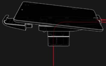
7. Squeeze the tablet into the clamp with the charging cable running behind the tablet.
