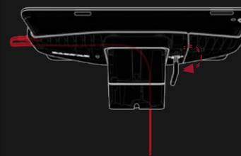
9. Remain holding clamp together until you have rotated the security lock with the L shape key into the lock position.
