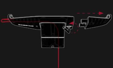
6. Unlock the security lock with the L shape key and slide the clamp out.
