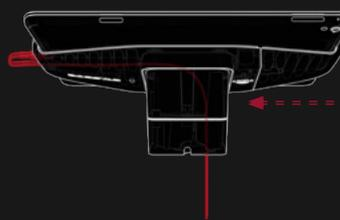
8. Re-attach the clamp arm by sliding in and squeezing tablet.
