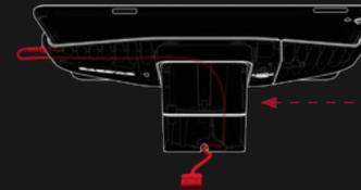
4. Re-attach the clamp arm by sliding in and squeezing tablet.
