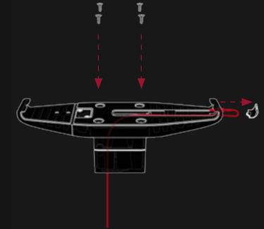
5. Remove the cable clip and place case back on the stand and screw back in the 4 screws.
