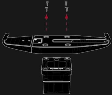
1. Unscrew screws and lift the Edge case off the stand.
