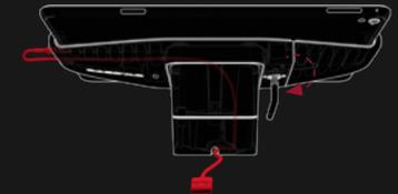
5. Remain holding clamp together until you have rotated the security lock in the lock position.
