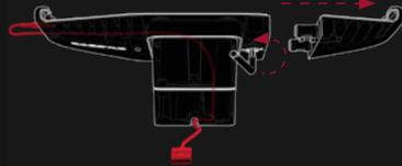
2. Unlock the security lock and slide the clamp out.
