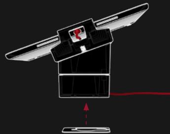
7. Stick 3M adhesive to the base of stand and firmly place down on your mounting surface. Let the stand sit for 24 hours before use.
