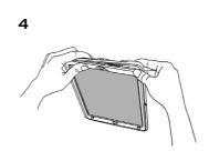
Reinstall the outer cover and press together to fasten.
