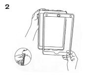
Pry the tabs slightly on each sides to unclasp the hard plastic frame.
