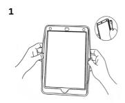
Peel off outer cover starting on arrows. Use the pick installation tool to assist.
